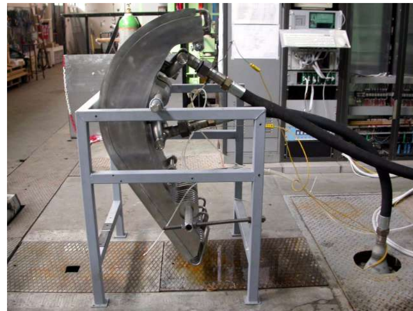
Hydraulic testing of IVT
